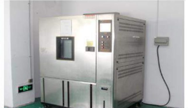
Constant temperature and humidity test chamber
