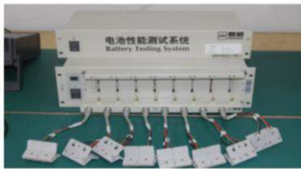
Battery performance test system
