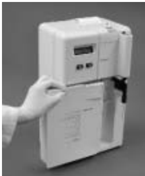
Pre-packaged reagents and waste reservoir in a plug-in, disposable pack eliminates sample contact and optimizes convenience.
