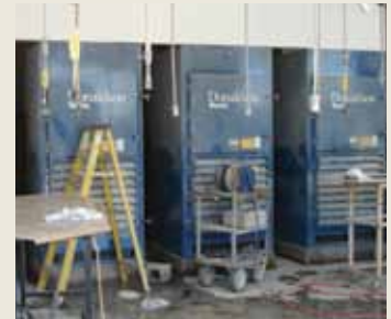
DWS Acabado de Granito 22,000 cfm
