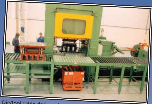
Die/tool table designed, manufactured and installed at Premier Spring and Presswork.
